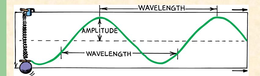
Electrons in the antenna of an AM radio station at 960 kHz vibrate 960,000 times each second, producing 960-kHz radio waves.
